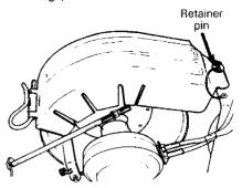
3. To remove the drive pulley guard, pull out the retaining clip (A) and pull on the spring (B) to disengage the pin from the bracket.
