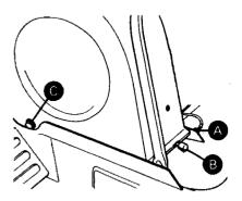
Push the pulley guard forward to disengage the front attachment (C) from the frame. Lift the guard from the vehicle.
