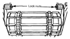
Adjust to proper tension by turning adjuster bolts clockwise to tighten counter-clockwise to slacken. Adjust both side equally.
