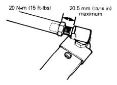
Handlebar should also be horizontal when the skis are pointed toward the front. To adjust; loosen the lock nuts of the shorter tie rod. Turn the tie rod manually until the handlebar is horizontal. Retighten the lock nuts firmly. Check tightness of the steering arm locking bolts and the wear of the ball joints.
