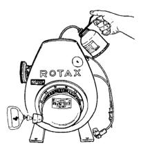
Slowly crank the engine several times using the manual starter.
