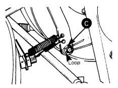
WARNING: Brake cable must make a loop around the bolt head. Strongly pull the brake handle to check cable tightness. Always check the brake light to see if it functions after performing brake adjustment.
