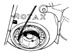
WARNING: After starting the vehicle in an emergency situation by the starting pulley do not reinstall the rewind starter assembly.
