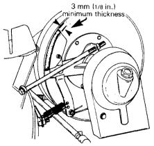
WARNING: Brake pad or puck less than 3 mm (1/8 in.) thick must be replaced. Replacement must be performed by an authorized dealer.
