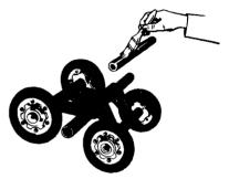
Grease each set then spray the springs with metal protector, or wipe with an oil soaked cloth. Assemble and install each set in the proper position.
