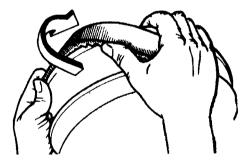
Slip the belt out from the drive pulley and remove completely from the vehicle. To install the drive belt, reverse the procedure.
